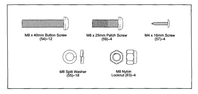
Identify the Front Stabilizer (15). While another person lifts the front of the Frame (1), attach the Front Stabilizer to the Frame with four M8 x 40mm Button Screws (54) and four M8 Split Washers (55).
